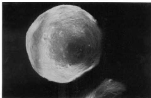
Fig. 2. Structural texture of dual coated microcapsules (magnification, 60\times ).
